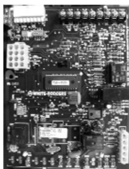
Integrated Ignition Control
